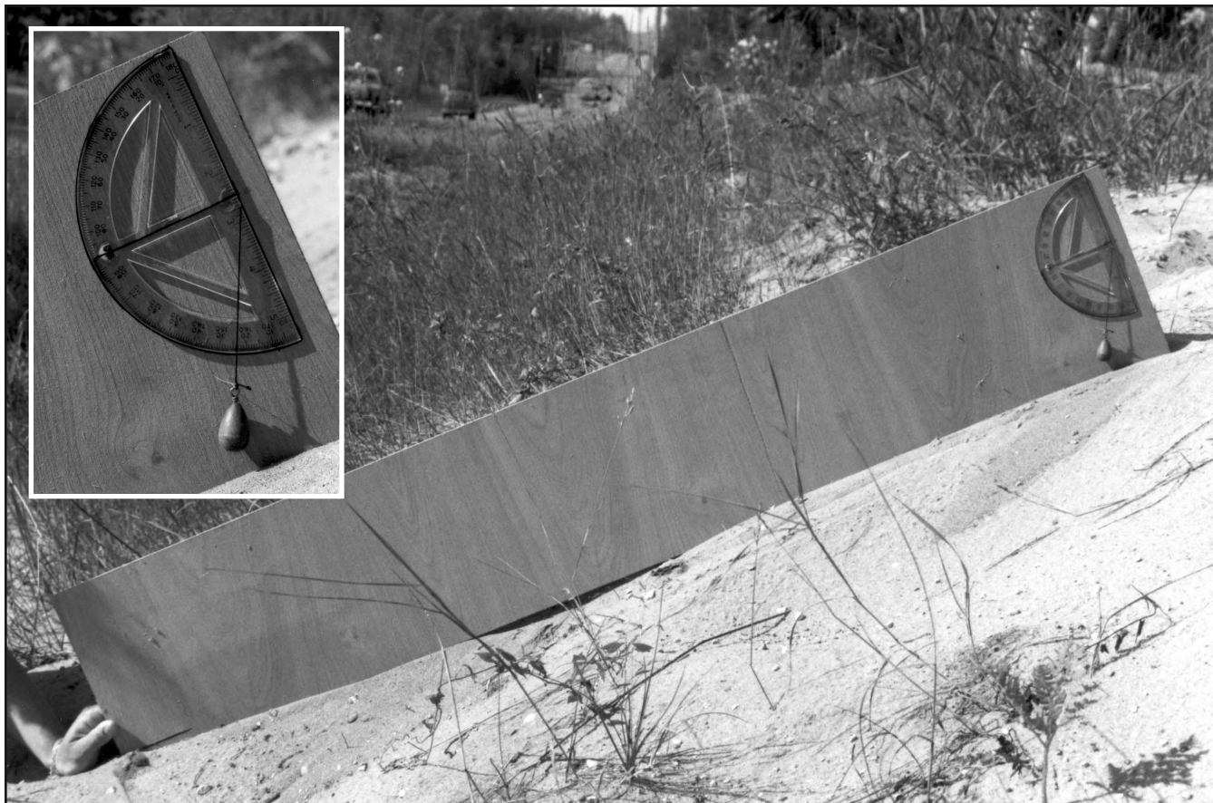
Figure 14: Determining the slope of a site targeted for erosion control. A 1:1 slope has an angle of 45^\circ , 1:1.5= 33^\circ , 1:2= 27^\circ , and 1:3= 18^\circ .
